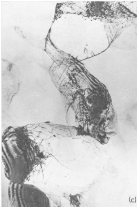
Figure 4 Development of the substructure in aluminium during annealing at 150° C. (a) Before annealing; (b), (c), (d) quenched after 5, 30, and 120 min respectively at temperature.
